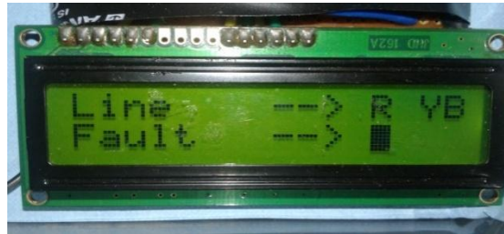
FIGURE 5.2 Fault In R-Phase
